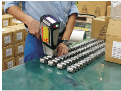
▲ 手持式分光分析儀 POSITIVE MATERIAL IDENTIFICATION (PMI)
